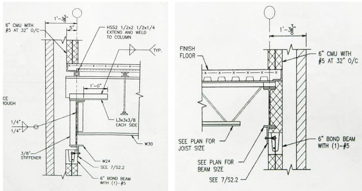
Figure 7: Typical Floor Section showing beam and columns relationship
