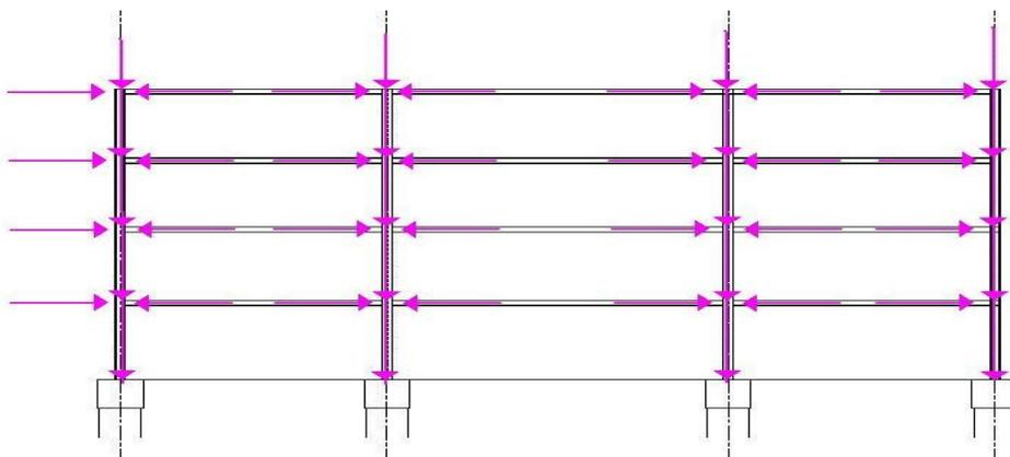
Figure 14: Lateral Load Distribution on the Frames
