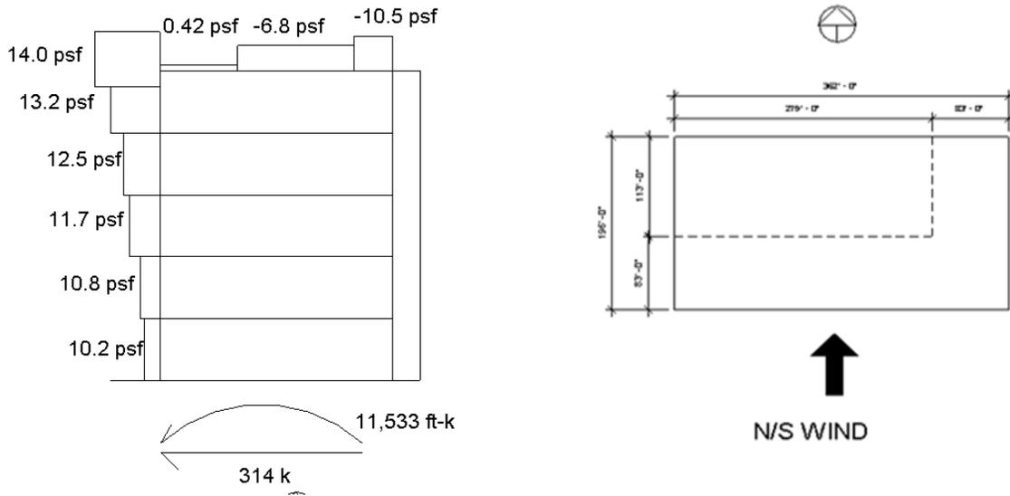
Figure 15: Wind Pressure diagram
