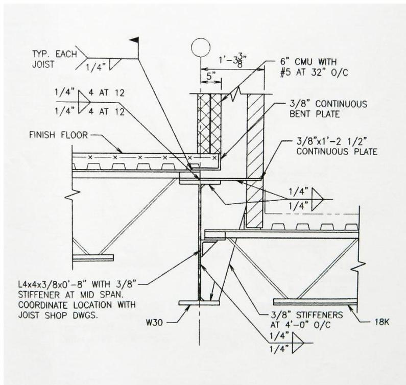
Figure 8: Joists and beam interaction
