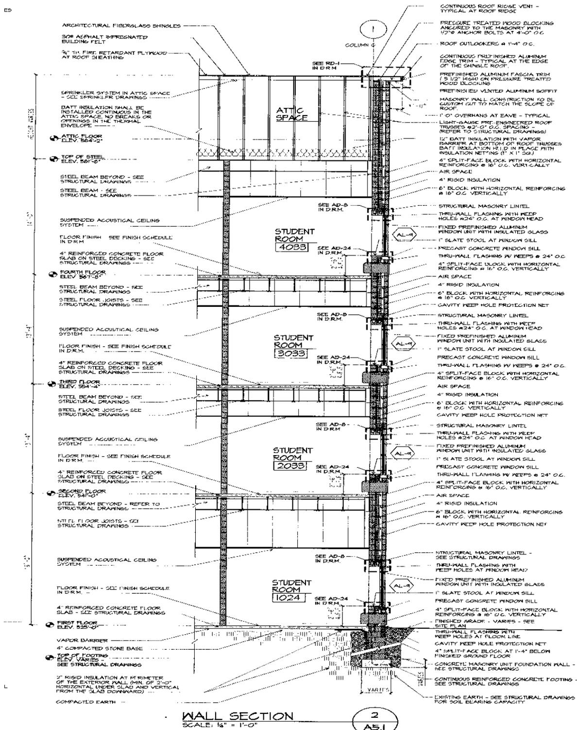
Figure 9: Wall Section
