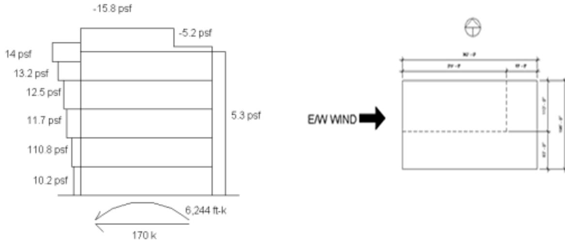
Figure 16: Wind Pressure diagram
